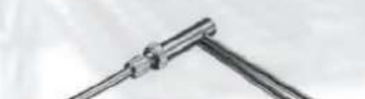
312.330 Insert Drill Sleeve with stop, for 4.5mm screws adjustable length to limit drilling depth, external dia. 4.5mm for drill bits of 3.2mm dia.
