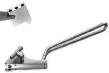
332.010 1 Triple Drill Guide 130° angle, for 130° angled blade plates and for condylar plates, drill bit 4.5mm dia.
