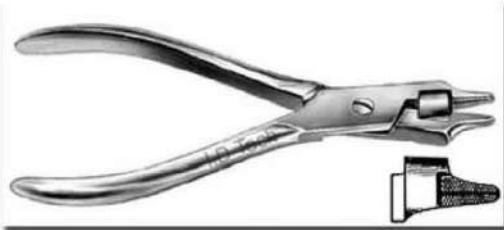
22-209-15 Combi-Flat Nose Pliers 15 cm / 6" for Bending & Cutting
