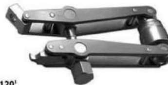
321.120 1 Tension Device, articulated Span 20mm, can also be used as a distractor. Colour scale: yellow up to 500N, green up to 1000N, red above 1000N.
