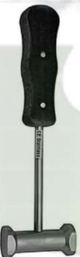
22-535-23 Fibre Handle Mallet 23cm / 9" Head Dia 30mm/Weight 12 oz. (340gm) Also Available in: Head Dia 35mm/Weight 1lb 40 oz. (570gm) Head Dia 40mm/Weight 1lb 90 oz. (708gm)
