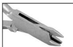
34.2191 Aderer, small Wire bending and loop forming pliers ● 0.36 mm to 0.50 mm (.014" to .020") ■ Max. 0.53 mm x 0.64 mm (.021" x .025")
