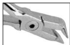
34.2127 Cinch Back / tie back Distal end bending pliers ● 0.30 mm to 0.50 mm (.012" to .020") ■ Max. 0.56 mm x 0.71 mm (.022" x .028")
