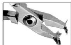
34.2128 Hammer head Distal end bending pliers ● 0.30 mm to 0.50 mm (.012" to .020") ■ Max. 0.56 mm x 0.71 mm (.022" x .028")
