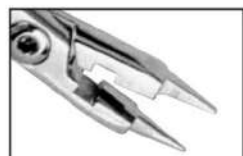
34.2126 Multi-purpose pliers, bird beak, De la rosa and cutter in one ● 0.30 mm to 0.50 mm (.012" to .020") ■ Max. 0.46 mm x 0.56 mm (.018" x .022")
